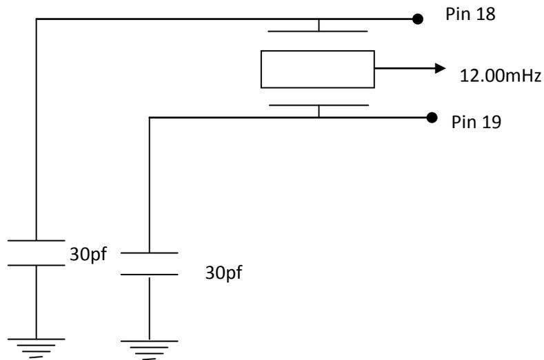
Fig. 3.8: Crystal oscillator unit
