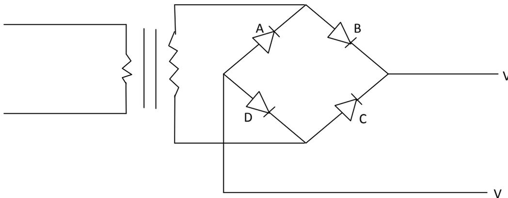
Fig. 3.11: Bridge rectifier
