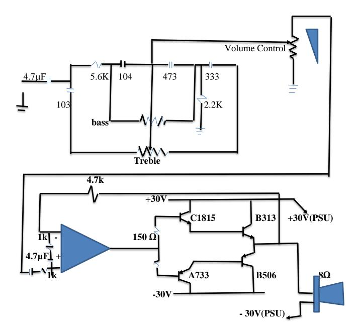
Fig. 12: Tone control circuitry connected to the amplifier.
