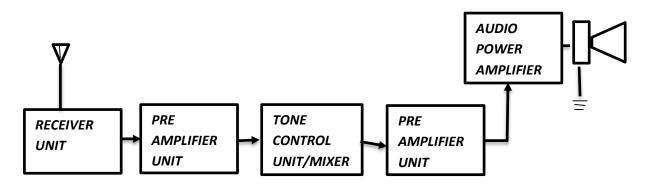
Fig 5: A block diagram of a receiver system
