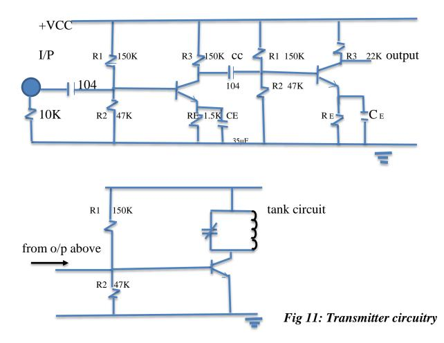
*Tank circuit*: This was used to generate the radio wave which is also a culprit design. This circuit generates radio wave by charging and discharging the capacitor. The capacitor charges through the coil at first half cycle and discharges through the coil in another half cycle forming a damping resonance frequency.
