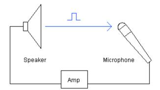
Fig.14 : public address system with acoustic feedback.
