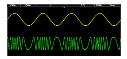
Fig 7: A typical FM shown with the modulating signal
