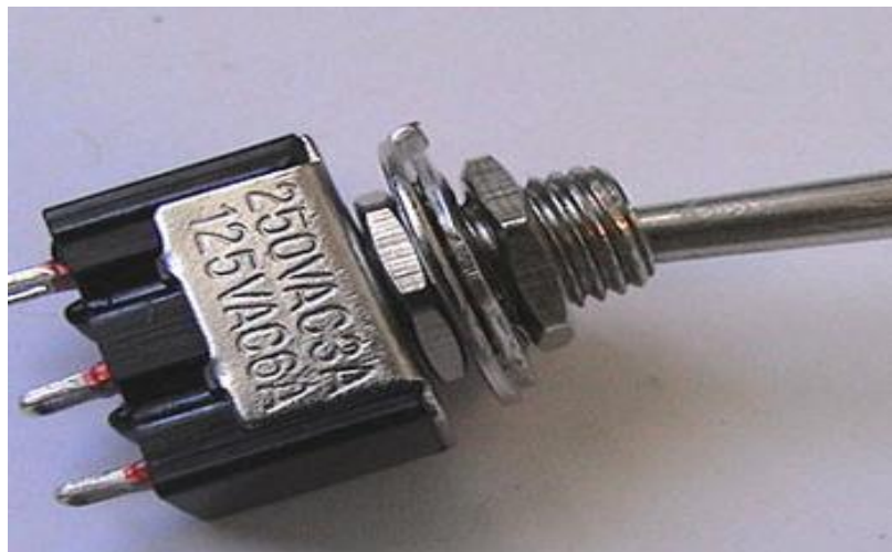
FIG 3.13. A TOGGLE SWITCH
