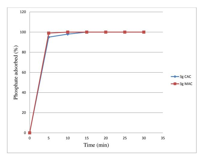
Fig 4.9: Comparison of adsorption rate of 1g of chemically activated carbon & microwave-synthesized activated carbon
